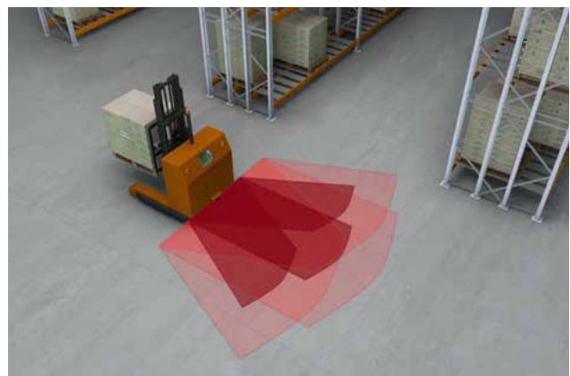
Flexible adaptation of the protective fields with automated guided vehicles (AGVs)
